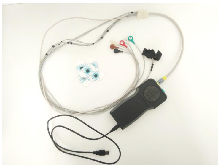
Fig. 2 Biotelemetric VLV-LAB system with disposable surface electrodes
