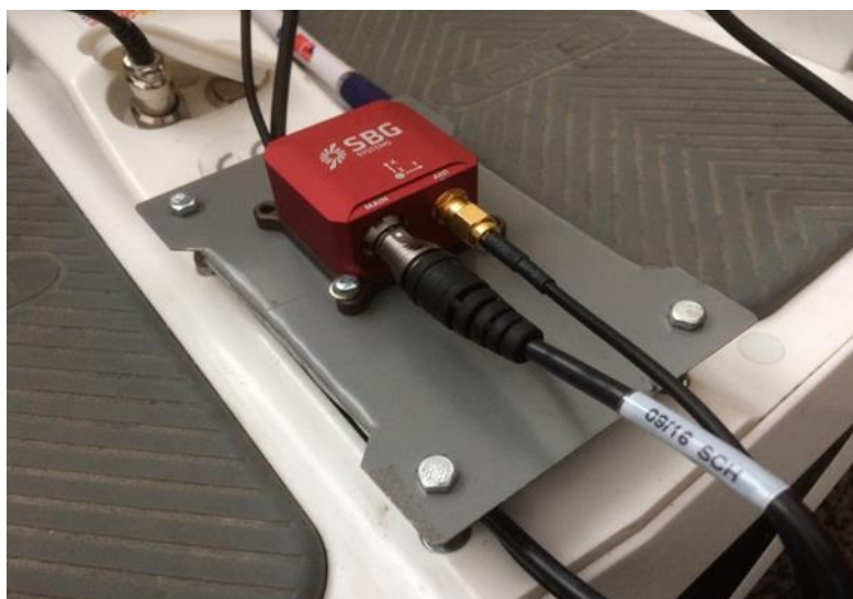
Fig. 2 Detail of the inertial unit attachment
