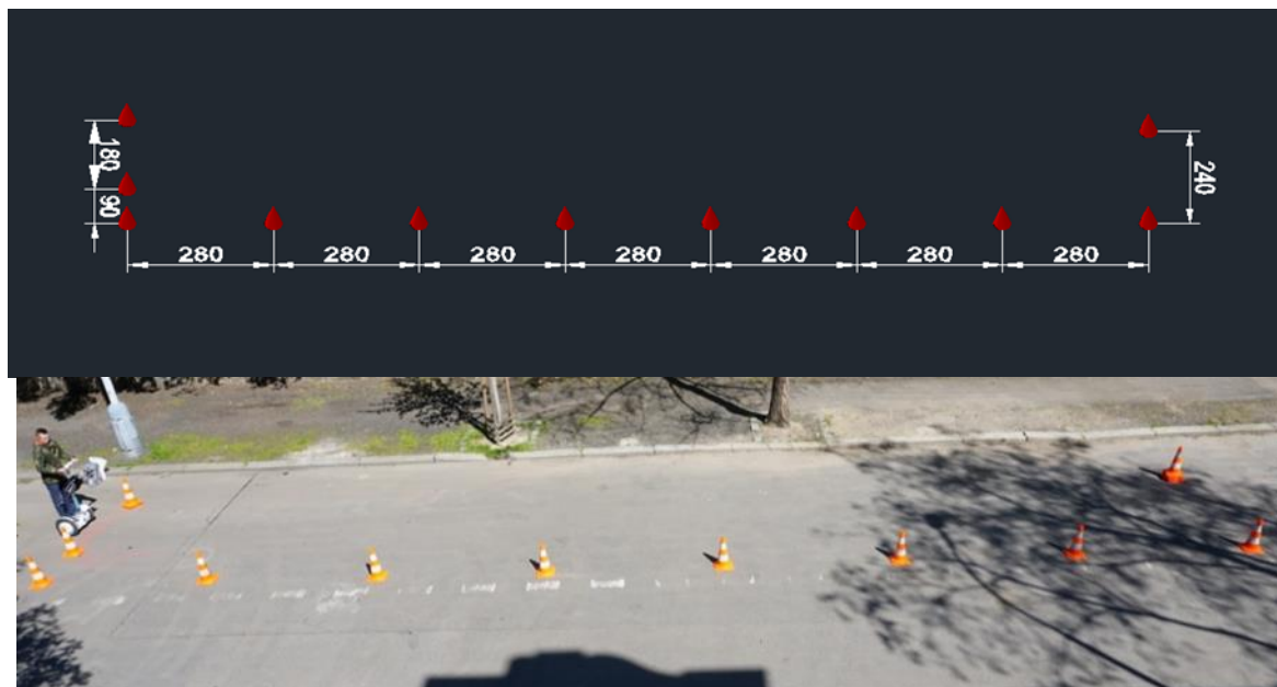
Fig. 3 Drawing of the trial track and photo of the track with rider at the start
